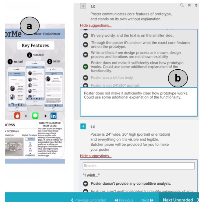
Figure 3. CritiqueKit implemented as a browser extension in Gradescope for DEP 1. a) Reviewers provide feedback on a student design. b) The suggestions box under each rubric item provides reviewers with a list of reusable suggestions and a comment box for providing feedback on a submission.
